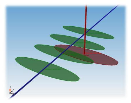
The following diagram shows the separation between each Reference Ellipsoid and the Offset Ellipsoid using the Pedal Curve method to calculate the separation. The report shows the separation between  $R_{4080m}$  and  $O_{3439m}$  is -42.78m. We can measure the distance using the measurement tool in the KellyDown Visualiser to see that the actual overlap is approximately -9m.
