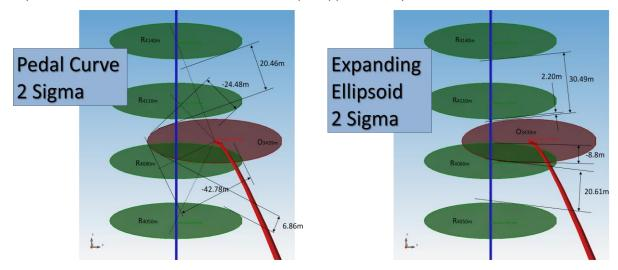
Similarly, the Pedal Curve method shows the separation between  $R_{4110m}$  and  $O_{3439m}$  is -24.48m, but we can see in the Visualiser that the ellipsoids are not overlapping and if we measure the distance in the KellyDown Visualiser, we see the separation is actually about +2m.
