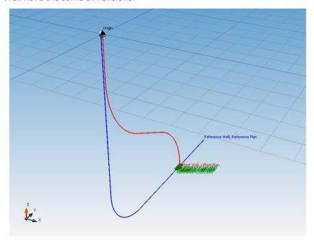
The Reference Well was scanned at regular intervals for proximity against the Offset Well and the measured depths of the four closest stations to the Offset Well were noted. Elliptical targets representing the four uncertainty ellipsoids on the Reference Well were created at each of the measured depths. An elliptical target was also created to represent the Error Ellipsoid at the bottom of the Offset Well.
